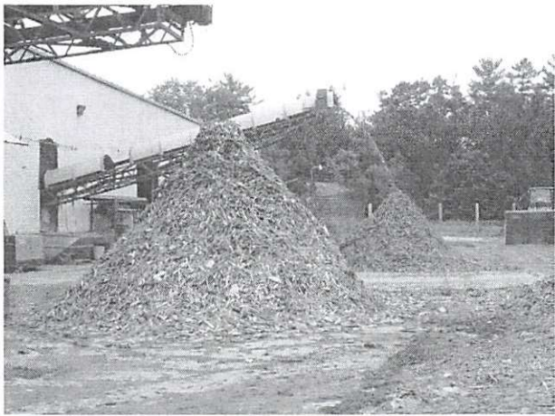
This C&D wood waste has been processed into a recyclable material, for use in manufactured wood products such as chip board.
