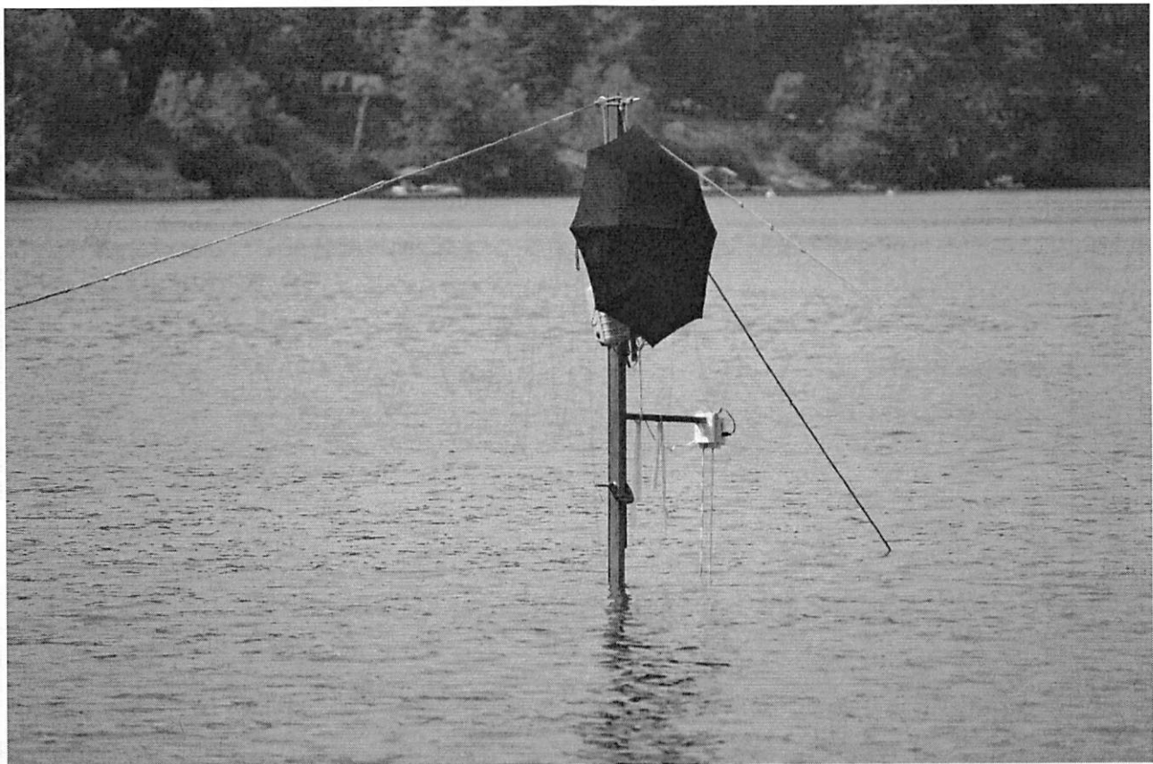
Figure 7 Photograph of the wave probe set-up
