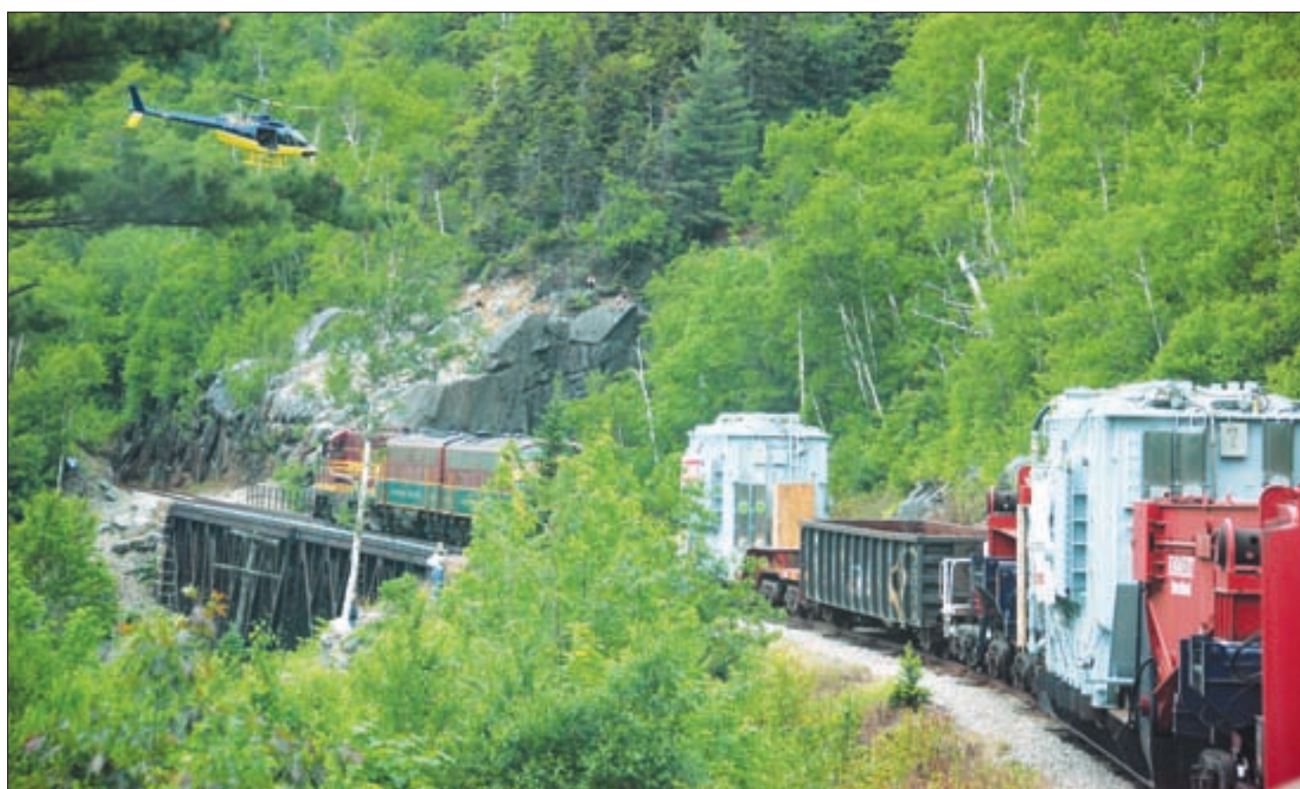
Three diesel electric locomotives, on the bridge, powered a special Conway Scenic Railroad (CSRR) freight train hauling a $9 million 411-ton electrical transformer on Saturday in two sections over the Willey Brook Trestle in Crawford Notch. The smaller 184-ton section is closest to the locomotives. Next, hitched behind an empty boxcar, is the larger 227-ton section carried on a Schnabel BBCX-1000 rail car, designed to suspend its oversized cargo between its two ends, making the load an integral part of this extra-long piece of equipment. The Heartland Media crew rides overhead in a helicopter photographing the unique journey for PSNH, which ordered the equipment for its Saco substation in Conway. (Photo by Edith Tucker)
